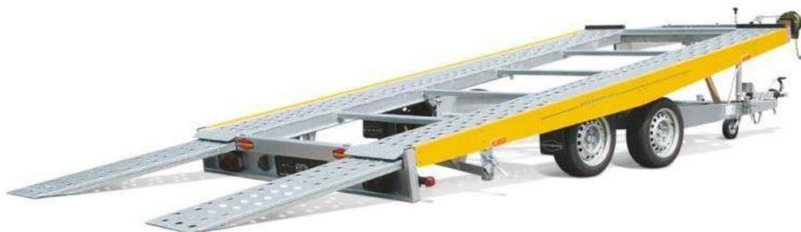
AH 4220/35, 430 x 208cm, Kippvorrichtung mittels Handhydraulikpumpe
